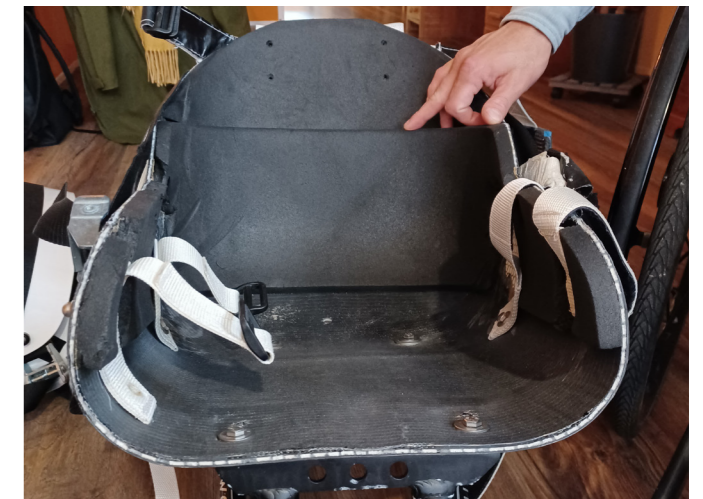
Figure A-5.10: front view of seat showing the curved edges around upper legs
