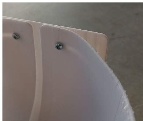
Figure C-2.6: prototype critical spot for lines getting stuck
