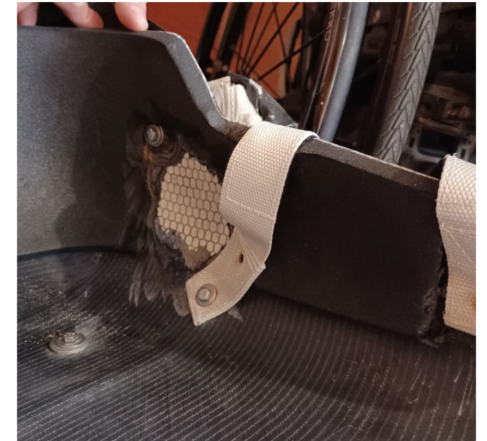
Figure A-5.5: Kite seat Willem Hooft with cut-out foam + carbon for tighter fit
