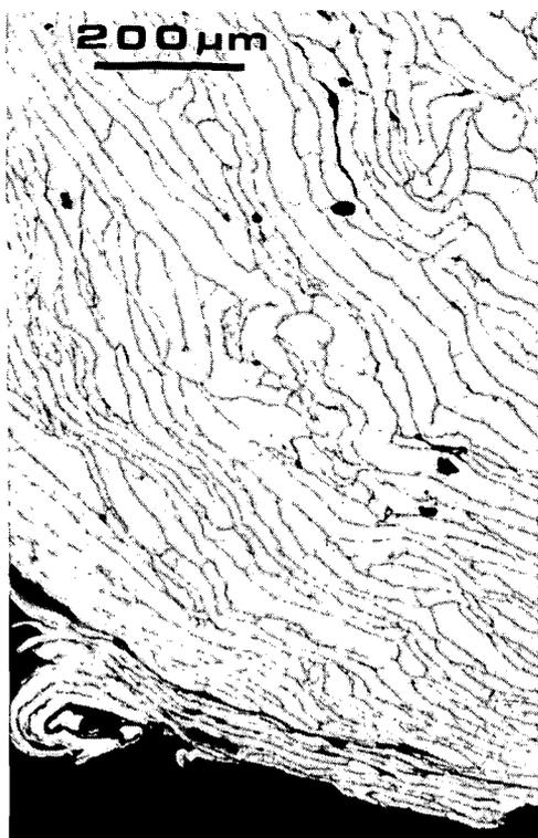
**Fig. 5a.** Transverse section of initial part of extrudate showing poor bonding between ribbons. Uncanned precompacted AlMg (2.3 at% Mg) ribbons extruded with an extrusion ratio of 44.4; optical micrograph.
