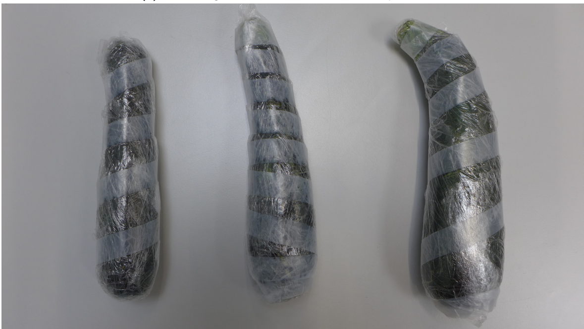
(b) In order to prevent damaging the system, the courgettes were wrapped in plastic foil.
