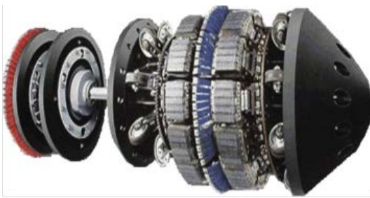
Fig.2 A magnetic flux leakage (MFL) pig[1]
