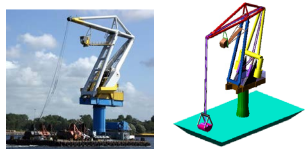
Fig.12 A floating lemniscate crane (Left: Picture; Right: Virtual MBD model)[23]
