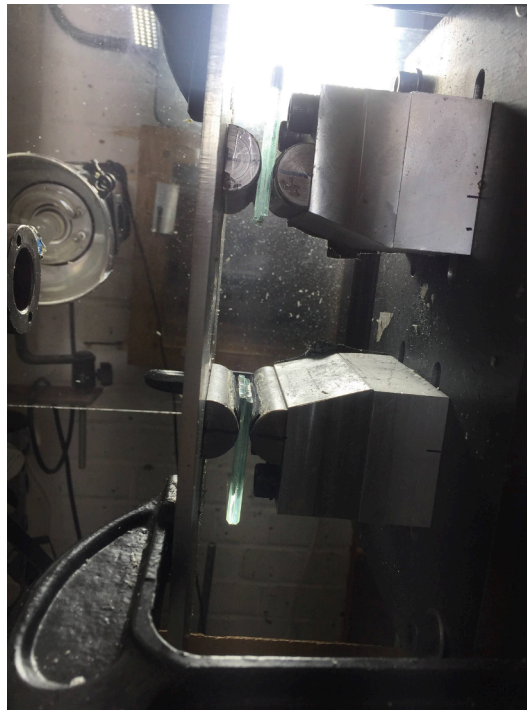
Fig. 19. Side view of the pinned supports providing axial restraint to a pre-fractured CS1 glass specimen (test type H) after impact with the polymer projectile.
