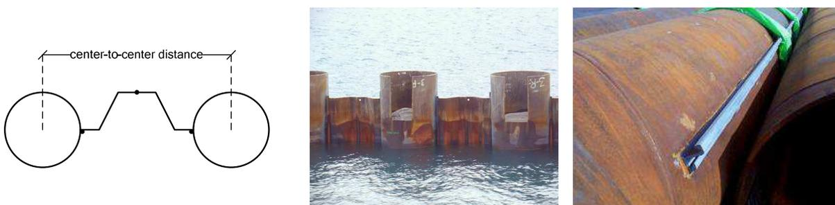
Figure 39-20 Cross-section, side-view and welded interlock of a combi-wall
