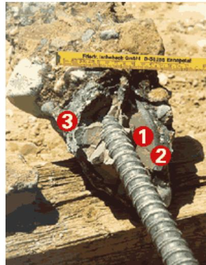
Figure 41-2 Installation of self-drilling grout anchor. (<http://www.ischebeck.de>)
