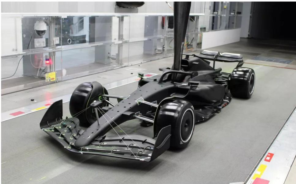
Figure 3.1: Formula One windtunnel model on rolling floor [20]
