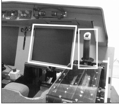
Figure 7. The manipulator and liquid crystal display (LCD) screen that were used for the experiment [12].
