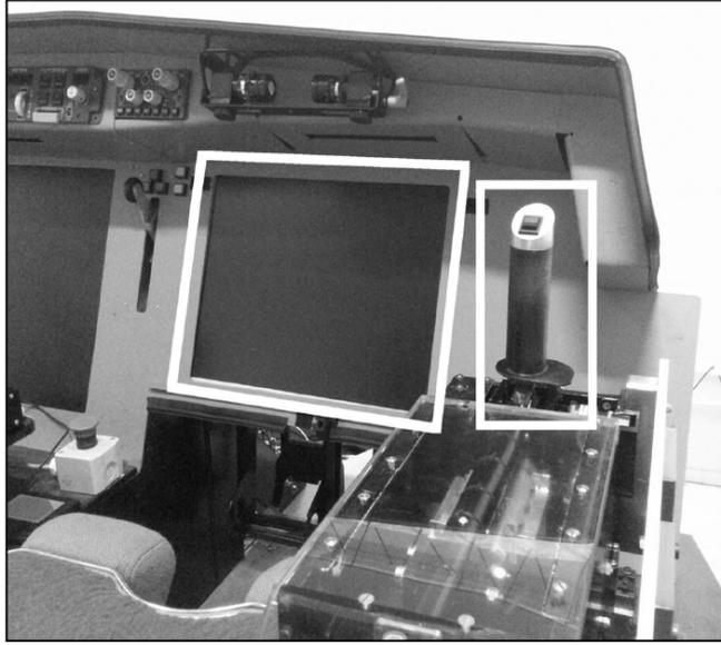
Figure 2.4: The LCD screen and manipulator used in the experiment [14].
