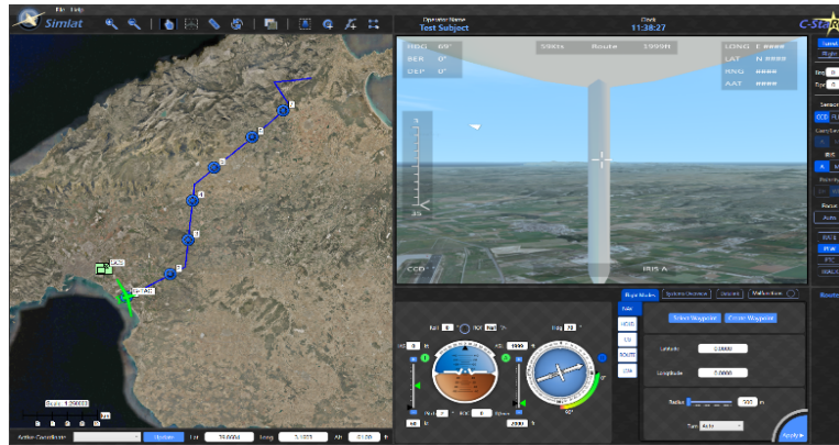
Figure 1. Trainee's Screen. Left side is showing the map screen with the route that the UAS will be following, while the right is showing the payload screen, with the zoom level indicator placed at the left edge of this screen.
