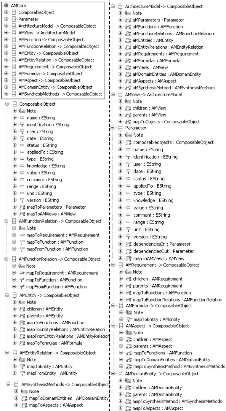
Figure 26. Class overview (top left), and specific class definitions in the architecture model. In the Eclipse / core class definition the 'class' icon indicates a class. The tree expanded under it shows its attributes.
