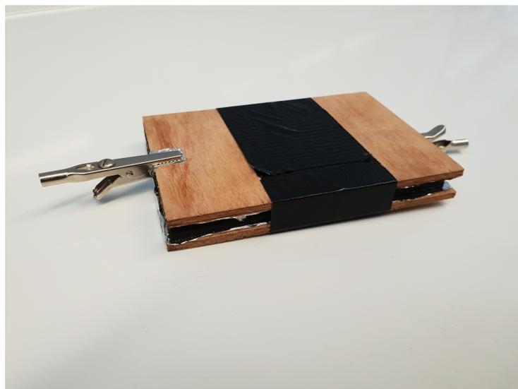
Figure 6.1: Parallel plate capacitor formed by two pieces of wood and aluminum foil
