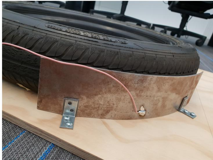
Figure 6.2: Wheel plate capacitor setup
