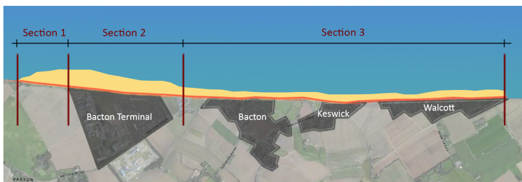
Figure 2.12: initial design. Sections are indicated by the red lines. Villages and Bacton gas terminal are marked in gray. The nourishment itself is marked in yellow.
