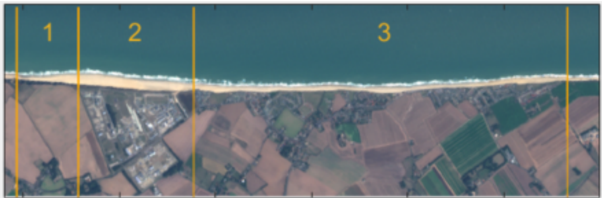
Figure 1: The feeder nourishment at the coast of Bacton. In yellow different parts of the nourishments are depicted. Number 2 indicates the area that is supposed to feed sediment to the adjacent areas 1 and 3.
