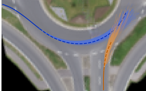
Figure 3.1: An example of the predictions generated by TrajFlow on the round dataset. Level of opacity indicates the likelihood of a given prediction.
