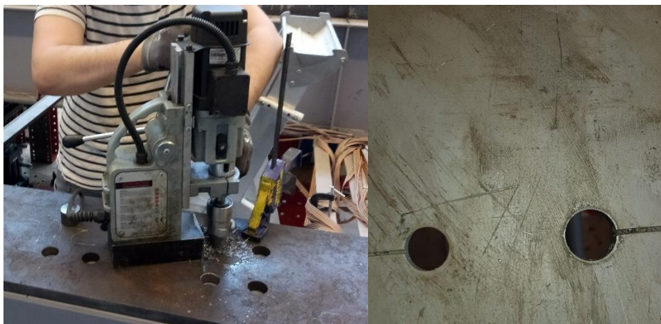
Figure 3.6 Hole size increase from Ø26 to Ø32 mm
