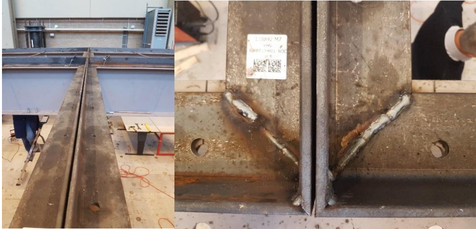
Figure 3.7 Welded L-profile frame
