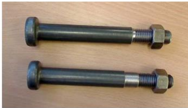
Figure 2.38 Threaded headed stud [59]
