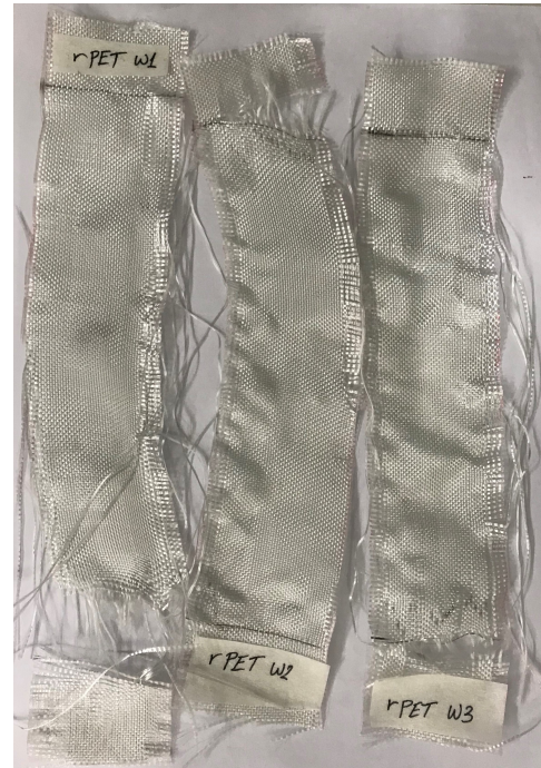
Figure 5.24: rPET W1-W3 specimens failure patterns
