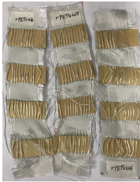
Figure 5.26: rPET SF W4-W6 failure pattern
