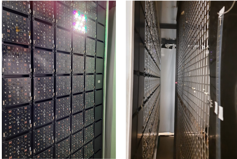
Figure 5.43: Float yarn test setup showing the solar wall (left) & the metal frame with the specimen attached (right).
