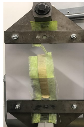
Figure 5.13: Specimen CY 7.5cm F2 after failure.
