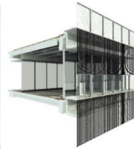
Figure 1.3: Double-skin textile facade - Rijkswaterstaat building, Utrecht, The Netherlands. [61]
