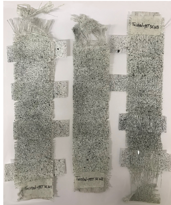
Figure 5.29: Twisted rPET SF specimens failure pattern.
