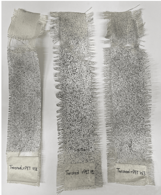
Figure 5.28: Twisted rPET specimens failure pattern.
