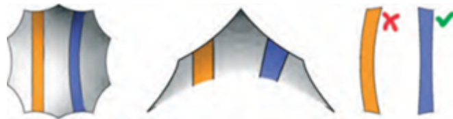
Figure 2.35: Cutting patterns following geodesic paths. [17]
