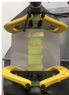
Figure 5.12: Specimen CY 7.5cm W1 after failure.
