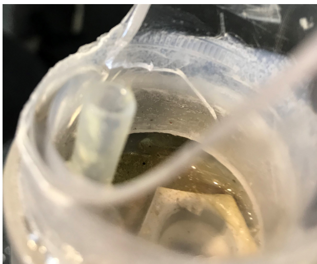
Figure 5.49: A close-up of the bottom part of the cracked degasser depicted in Figure 5.48, several small cracks and damage are visible
