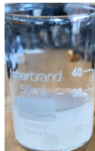
Figure 5.44: A sample taken from the liquid on the high pressure side. The white-grey colour originates from the formed aluminium hydroxide - Al(OH)_3 , an intermediate product of the corrosion of aluminium in alkaline media, pH 12.5
