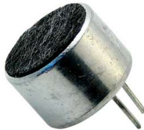
Figure 2.5 Electret condenser microphone
