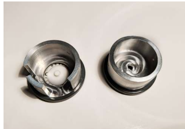
Figure 9.2 Stethoscope chestpieces designed and manufactured for testing the microphones
