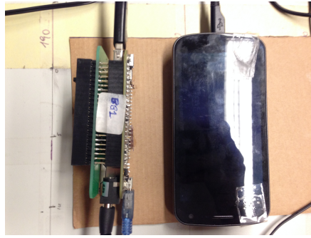
(a) Android Smartphone connected with a Beaglebone via USB cable.
