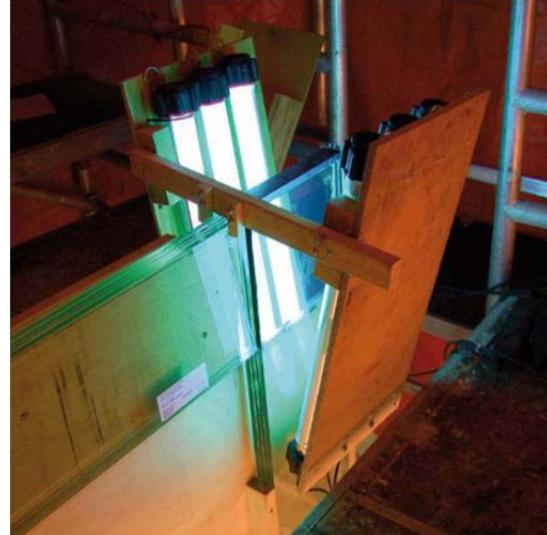
Figure 2-17 Manufacturing of the glued connection: application of adhesive (left), curing with UV- and visible light (right).(Weller 2010.)
