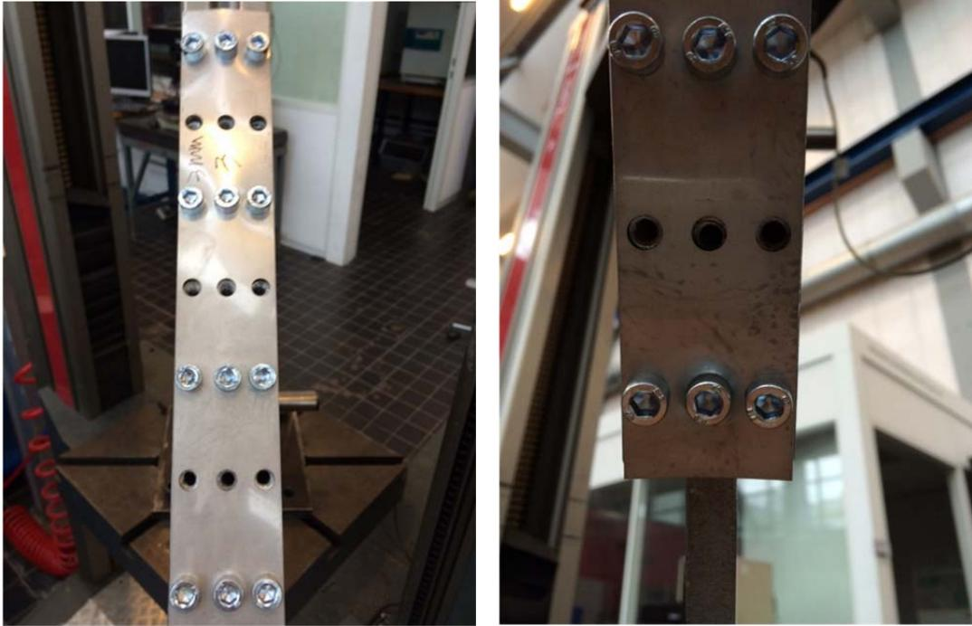
Figure 5-14 Deformation of the 3mm L-shaped connection (1) Upper side (2) Lower side
