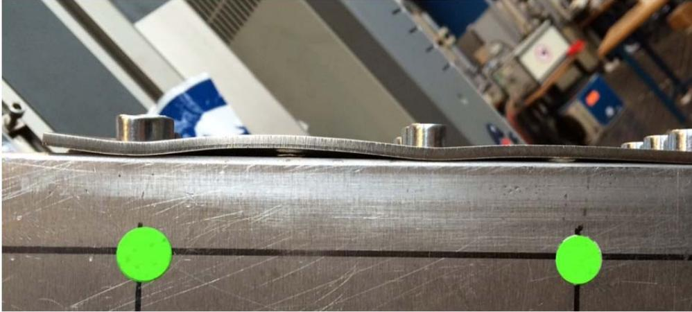
*Figure 5-18 Deformation of the 3mm L-shaped connection side view*
