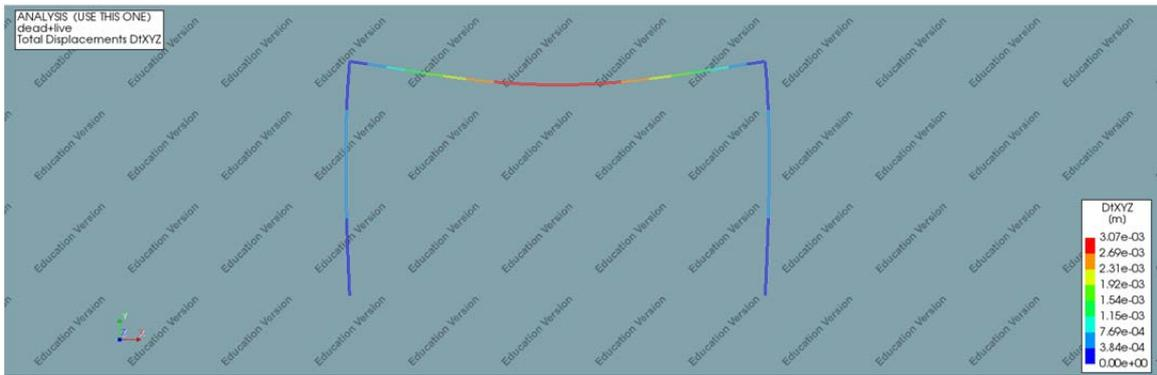
Figure 4-8 FEM analysis  $k=4000$ , deformation= $0.00307m$
