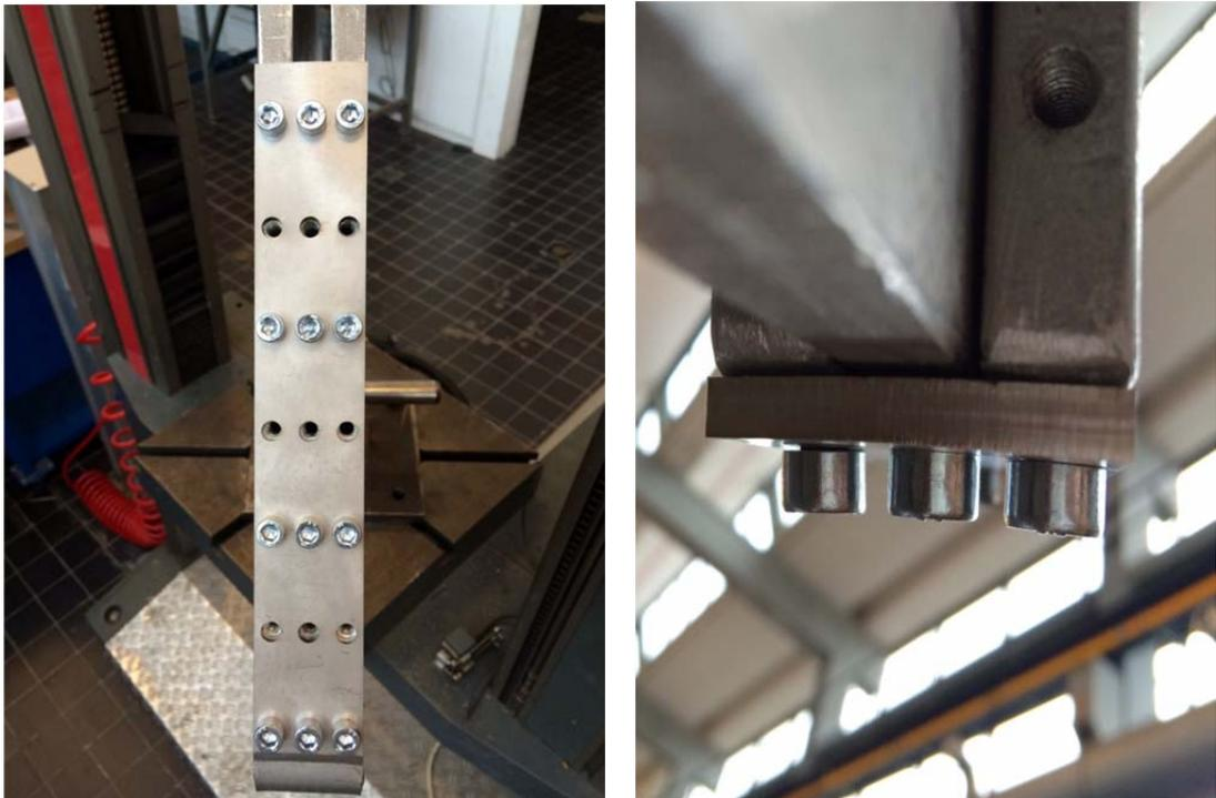
Figure 5-15 Deformation of the 5mm L-shaped connection pattern 1 (1) Upper side (2) Lower side
