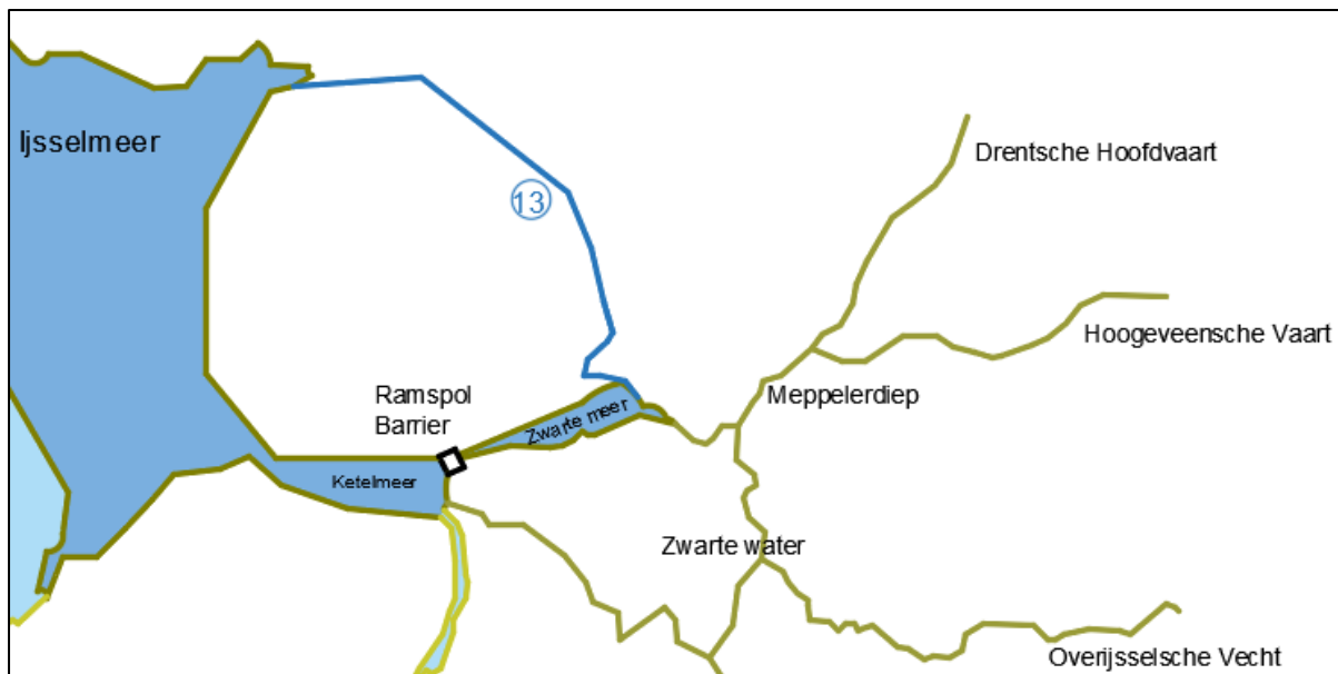
Figure 13 Improvement 13: Extension of Vollenhover channel to IJssel Lake (outflow discharge)
