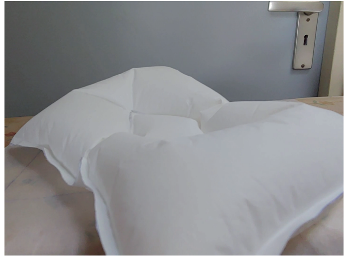
Figure A7: Inflatables were made by melting shower curtain in shapes using an iron.
