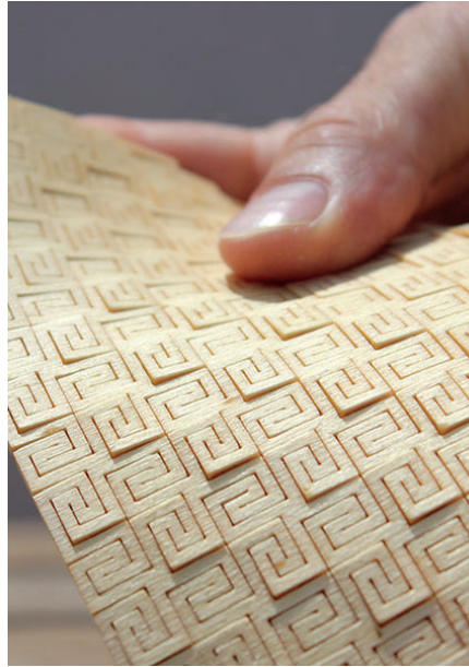
Figure 36: This laser-cut pattern allows wood to become double curved and flexible (image: kofaktorlab on Instructables).
