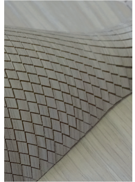
Figure 37: Wooden surface stretched by an airpocket below (image: AirWood by Arca).
