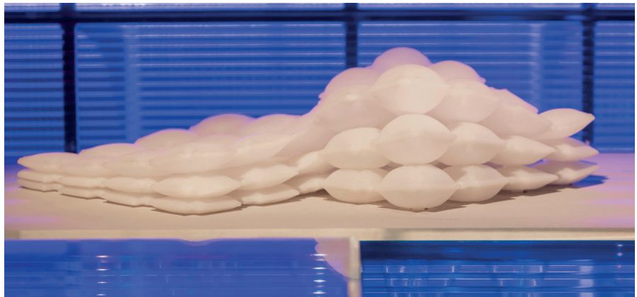
Figure 48: Liquid Printed Pneumatics allow for the creation of intricately shaped inflatables (image: BMW, in collaboration with MIT, youtu.be/vgz10_Kc0A0 ).
