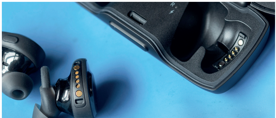
Figure 49: Wireless earbuds often use contact charging in a charging case (image: Soundguys).
