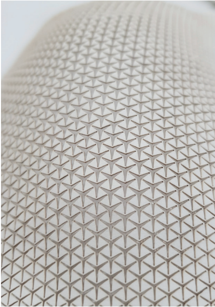
Figure 35: Cutting paper following auxetic structures allows it to be stretchable (image: Ben Street).
