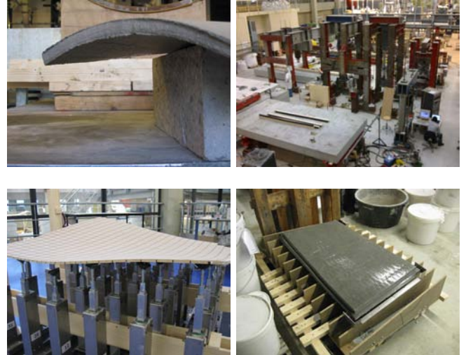
Figure 4. Experiments in the Stevin Lab with double curved precast concrete based on the patented system [8]
