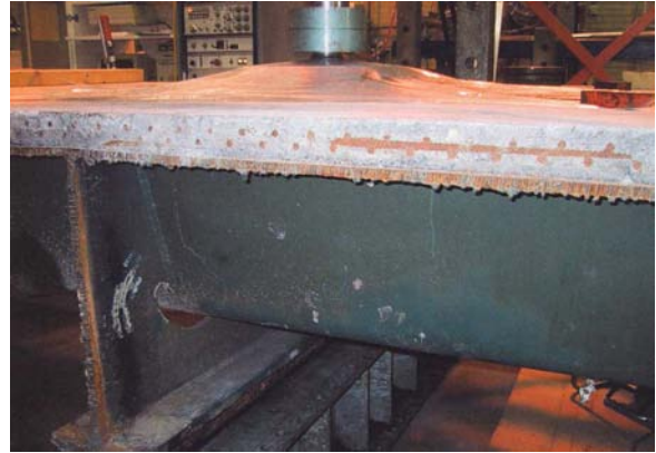
Fig. 11. Fatigue test on a bridge deck with high performance concrete.
