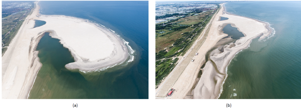
Figure 4.1.: Aerial photos of the SE, taken from the North, in a) July 2011 (shortly after construction) and b) July 2022 (after the first year). Source: Rijkswaterstaat and van Houdt (2012)
