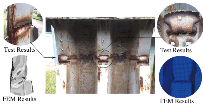
Fig. 14. Buckling failure of Specimen L1.
