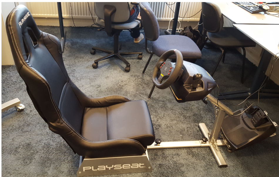
Figure 4.3: Driving simulator's hardware: vehicle seat, steering wheel and pedals.
