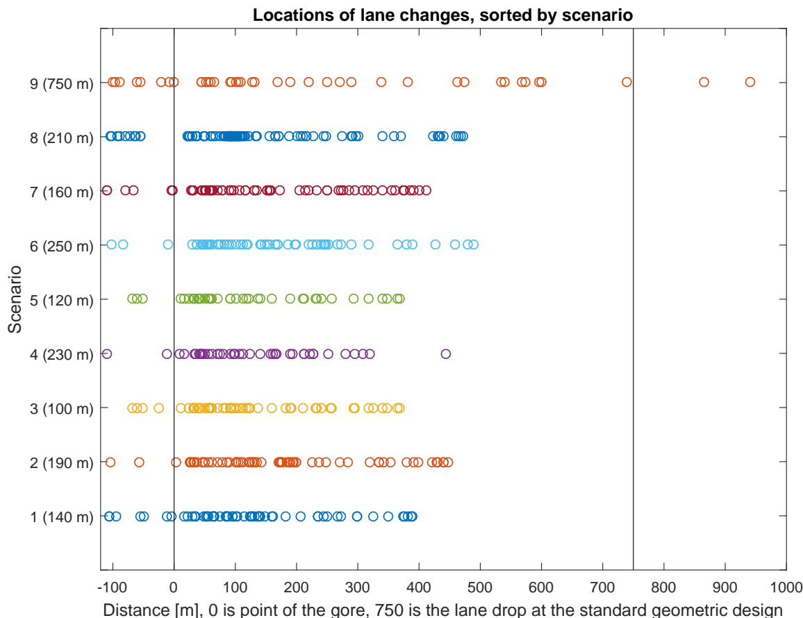
Figure 5.11: Lane change locations (in longitudinal direction) measured in the driving simulator, sorted by scenario.
