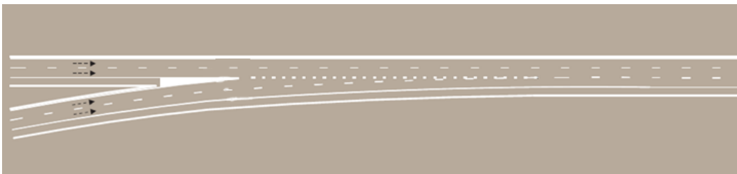
Figure 2.1: Schematic representation of the geometric design of a merging taper. [4]
