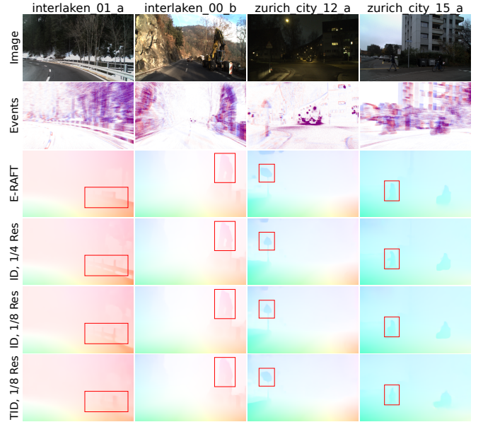
Fig. 4. Qualitative results of optical flow predictions on DSEC-Flow with highlighted regions of interest. Images are for visualization only, as optical flow is event-based. Test samples reveal that our ID method at 1/4 resolution produces superior results on fine details and small objects, while the TID method yields results that are comparable to those of E-RAFT.
