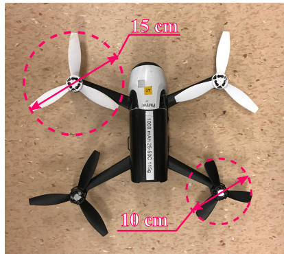
Figure 6.12: A Bebop 2 quadrotor with one damaged rotor.
