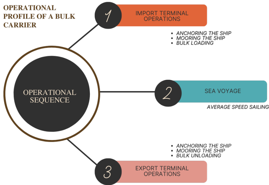
Figure 3-5: Sequence of operation of the Bulk Carrier
