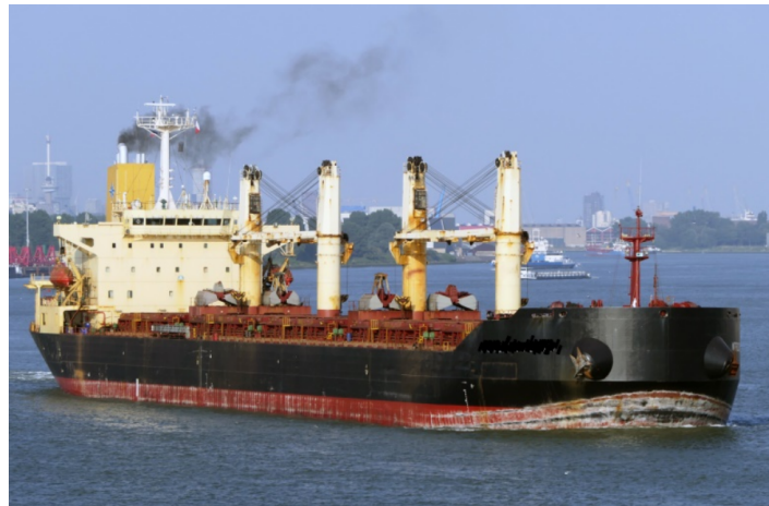
Figure 2-6: Handymax bulk carrier with 4 deck cranes [35].
