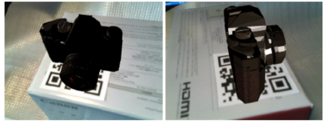
Figure 1: Example of QR codes and AR, showing a full 3D model of the camera [3].
