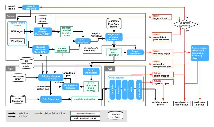
Fig. 3. Schema of Team Delft's sense-plan-act workflow for picking a product *X* from the shelf's bin *Y*. The sense step consists of: 1) detection of the target item and estimation of its 6-D pose, and 2) obtain collision information inside the bin, in the form of a PointCloud.
