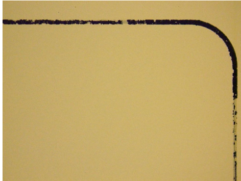
(a) Liftoff at 25°C temperature in a 60s NMP bath with 10 seconds of agitation.
