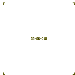
Figure 4-4: Mask for die labels and dicing marks on the back side of the top wafer.
