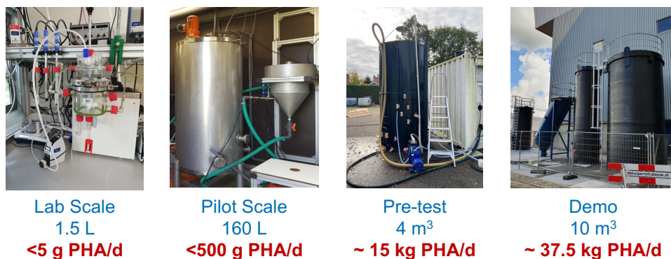
Figure 7.3: The volume of the reactors at different scales and the estimated PHA productivity. Photos by Ángel Estévez-Alonso, Erik de Vries, Paques Biomaterials BV, PHA2USE in the order of appearance.
