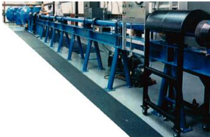
Figure 2.28: A two-stage light gas gun in use by the NASA hypervelocity impact technology facility. (Christiansen, 2006)
