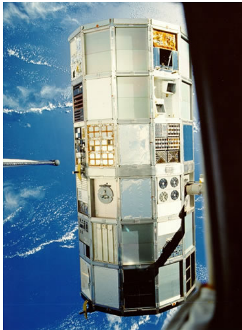
Figure 2.18: The Long Duration Exposure Facility (LDEF) in orbit after deployment from a Space Shuttle, clearly showing its surface experiments. (Stansbery, 2009)
