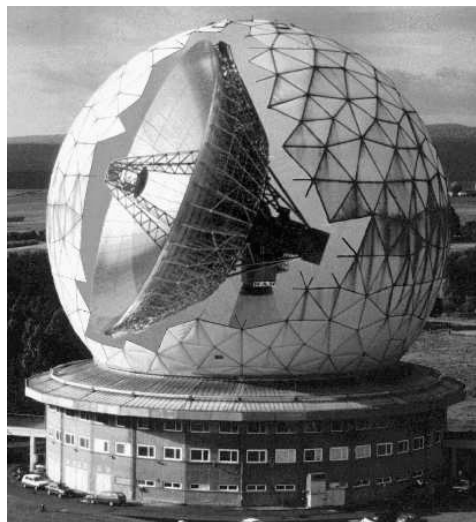
Figure 2.16: Artist's impression cutout of the main transmitting and receiving antenna of the TIRA system. (Klinkrad, 2006)
