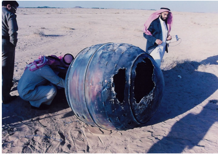
Figure 2.11: The remains of a decayed titanium motor casing of a Delta 2 rocket which landed in Saudi Arabia. (Stansbery, 2009)
