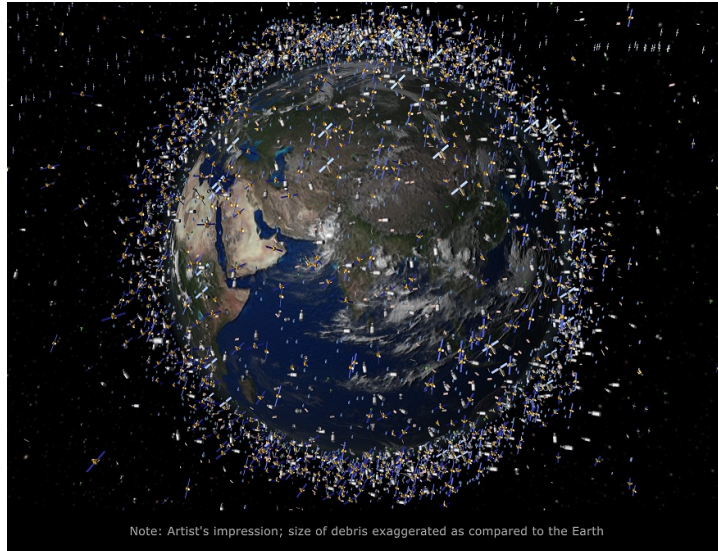
Figure 2.3: Depiction of the amount, type (rocket bodies and satellites are depicted differently) and spatial distribution of the debris with respect to the Earth for the LEO region. (Klinkrad, 2009)
