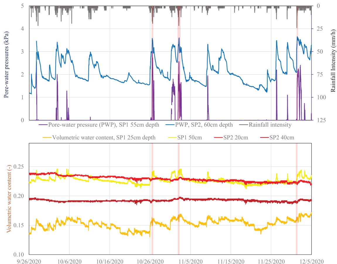
Figure 1. Time series of rainfall and pore water pressure and volumetric water content in two soil pits (SP1 and SP2) recorded on a steep hillslope above Sitka, in southeast Alaska, observed during a sequence of large storm events in October–December 2020 (dates in UTC); the days on which landslides occurred throughout the region are shown by the transparent red bars. Note that data are available for download in Smith et al. (2023), and near-real-time plots of data are available for situational awareness at https://usgs.gov/programs/landslide-hazards/science/sitka-ak , last access: 11 November 2024.
