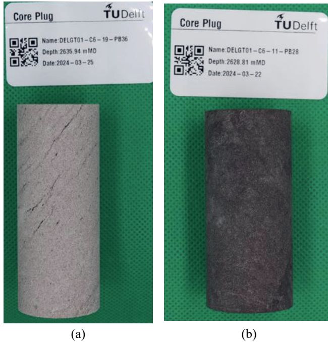
Figure 4.2 Core plug examples from the DEL-GT-01 wellbore: (a) sandstone and (b) shale.
