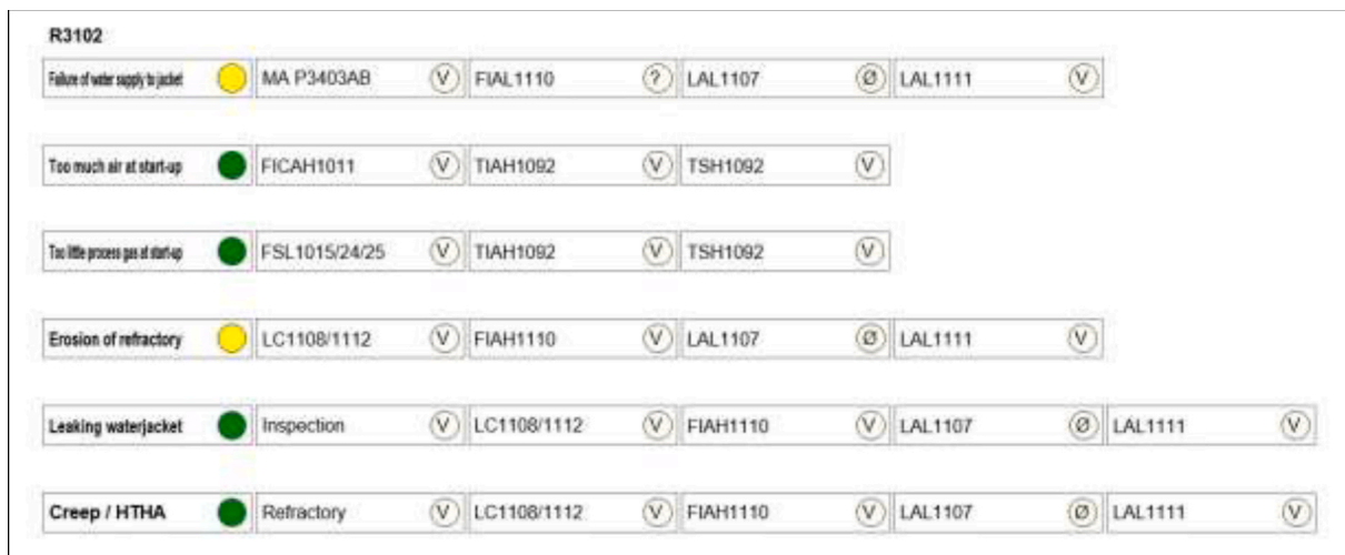
Fig. 9. Screenshot of the process safety dashboard of the post reformer.
