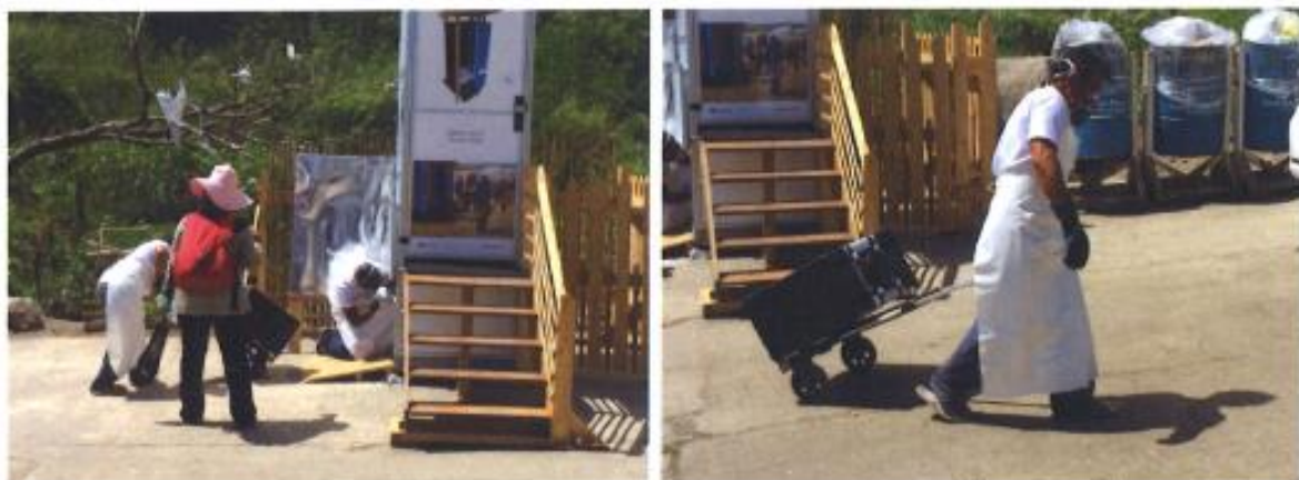
Figure 3-6 Evacuation of urine and feces tanks from experimental eSOS Smart Toilet during testing in Tacloban City, Philippines (Photos: F. Zakaria)
