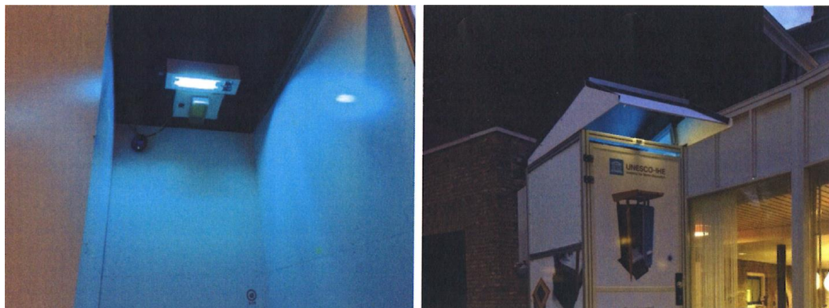
Figure 3-18 Activated UV lamp in experimental eSOS Smart Toilet during testing at IHE Delft (Photos: J. Curko)
