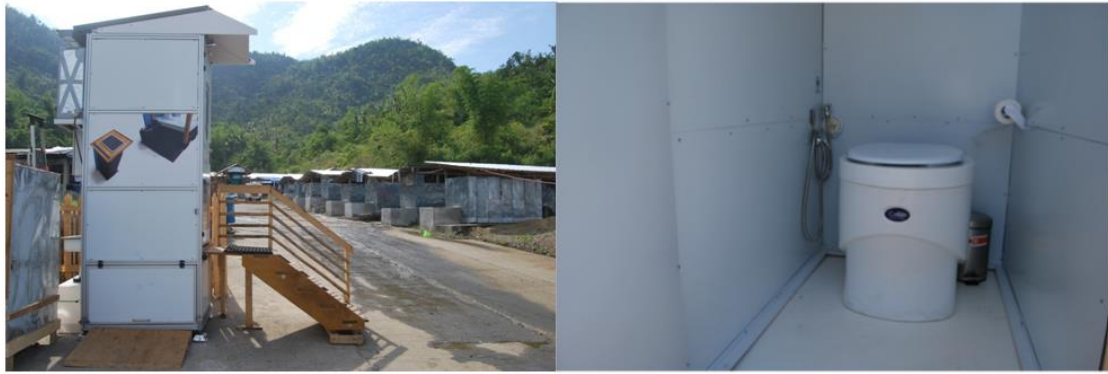
Figure 6-1 Experimental eSOS Smart Toilet at field test site in Tacloban, the Philippines (left); the interior (right) (Photos: F. Zakaria)
