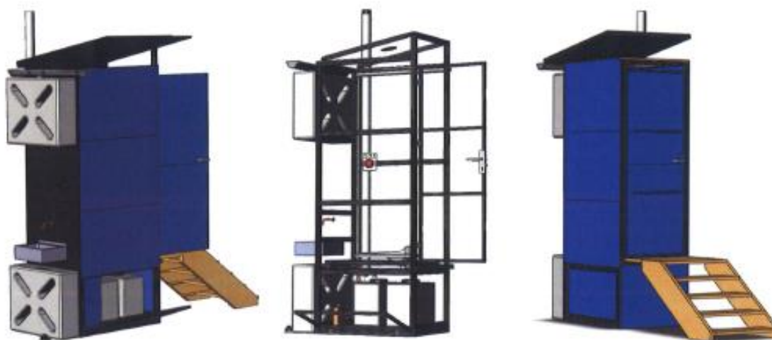
Figure 3-2 The conceptual design of the experimental eSOS Smart Toilet (Images: Flex/design)
