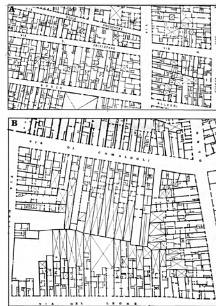
Fig 8. Florence's building survey at Santa Croce and San Frediano districts. Samples of medieval building fabrics. The underlying building tissue acts as the concept which is historically responsible of the fabric construction. The tissue expresses, at a specific level of complexity, named scale, the collective intentionality which establishes its set of rule, or its structure. The structure itself is questioned by modifications which constantly occur and can eventually lead to its transformation. The authors emphasize the material continuity of the process, uncritically assuming a continuity of values as well.
