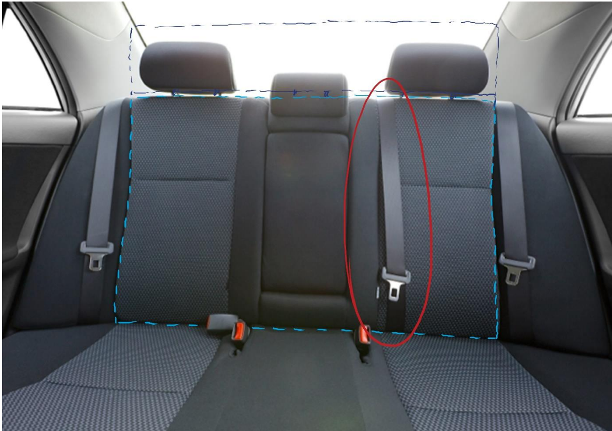
Figure R.1 The middle seat blocks the possible folding of a double backrest
