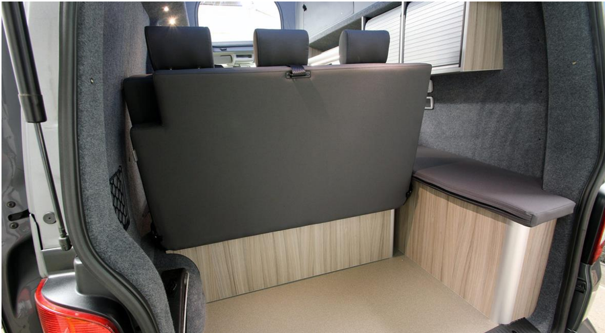
Figure K.8 The foldable cushion is attached to the back of the backrest
