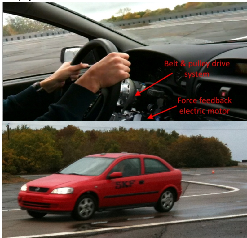
Fig. 7B 1. Force-feedback Opel Astra during test-track driving.
