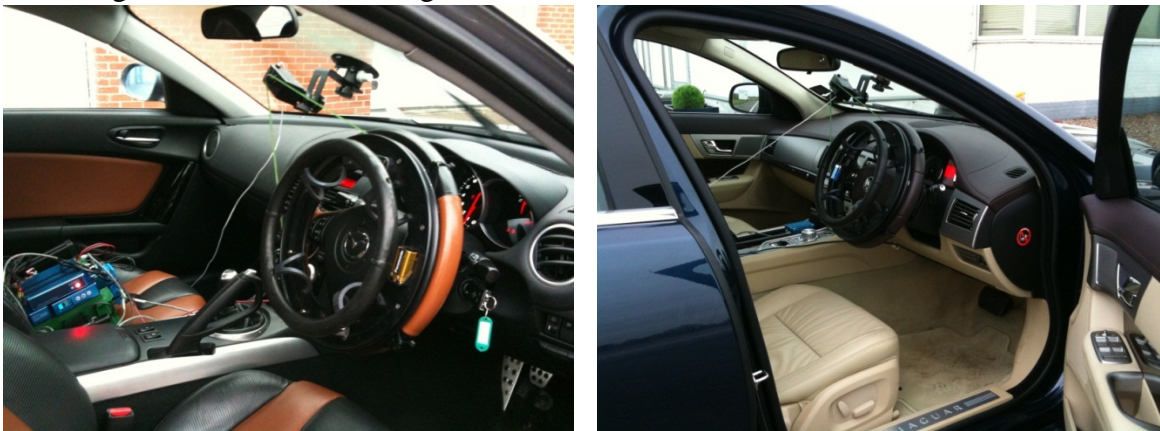
Fig. S 2. Steering indices measurement for different vehicle's in Prodrive, UK. Mazda Rx-8 (left), Jaguar XF (right).
