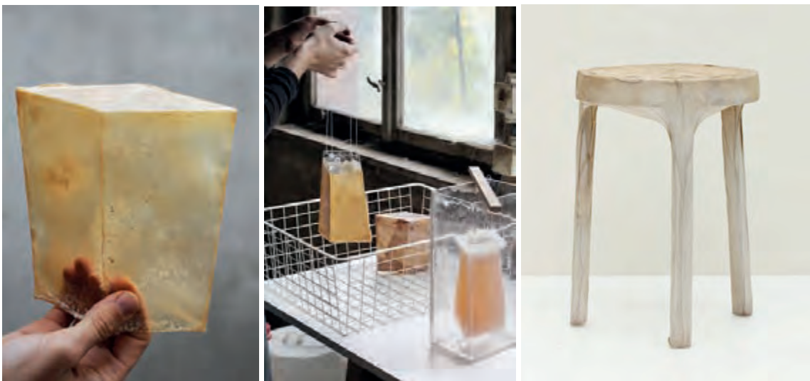
Fig 4. "Xylinum project" – growing bacterial cellulose directly in 3D complex shapes.
