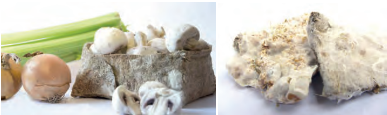
Fig 2. "The Factory of the Future" – a concept of sustainable packaging made from a mycelium-based composite, developed for the circular-economy-based farm 'Uit Je Eigen Stad'.
