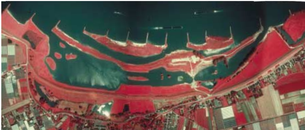
Figure 5.3 The Gamerensche Waard with three secondary channels (false colour aerial photo June 2000).
