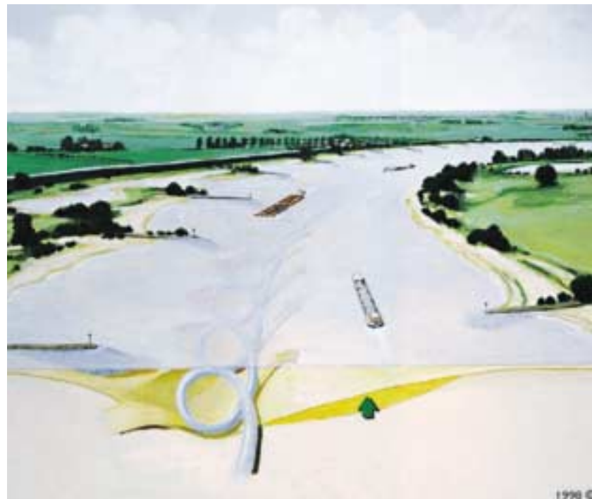
Figure 1.9 The spiral flow in a meandering river. (Schoor & Sorber 1998).
