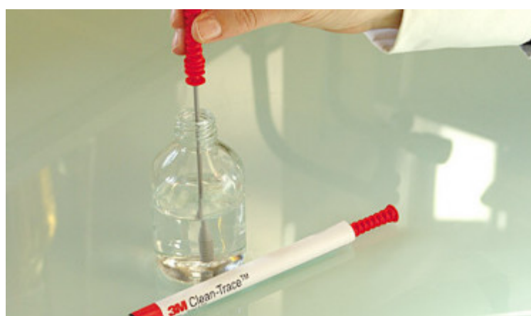
Figure 3.4: The measurement of tATP with the AQT200 swab of 3M
