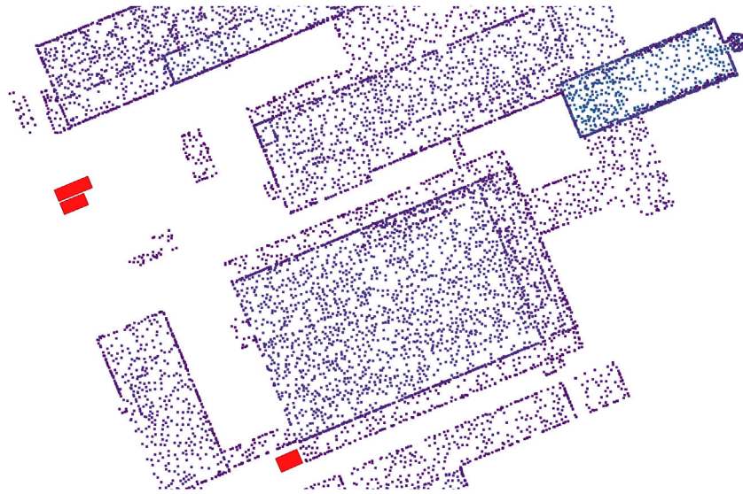
FIGURE 13 Failed reconstructions (in red) due to lack of elevation data.
