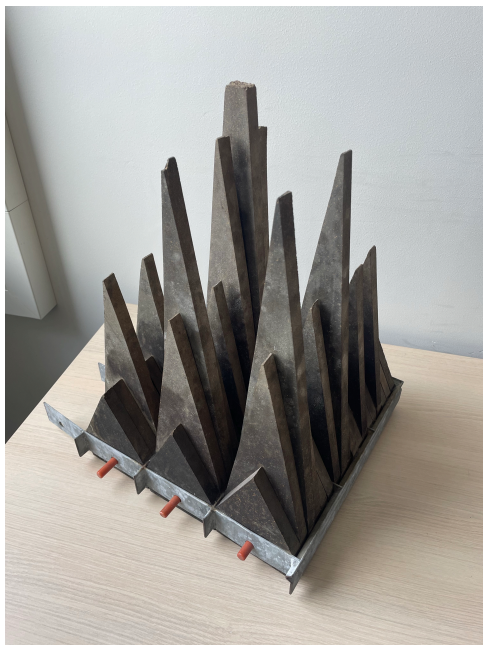
Figure 7.2.: Section of the anechoic lining mounted on the walls and floor of the basin. The lining consists of sound-absorbing pyramidal structures formed by stacked cork elastomer wedges.
