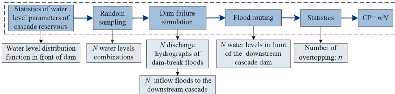
Fig. 10. Calculation of the CP of successive dam failure.
