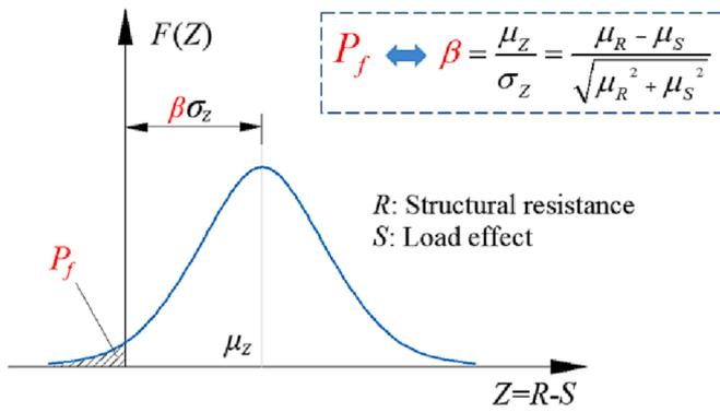
Fig. 3. Relationship between reliability index and failure probability.
