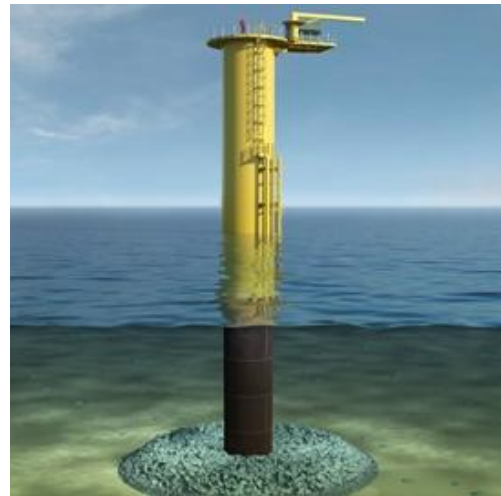
Figure 4, An offshore monopile foundation
