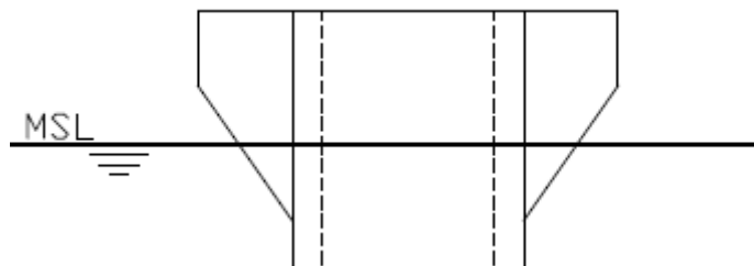
Figure 65, Ice cone layout for foundation
