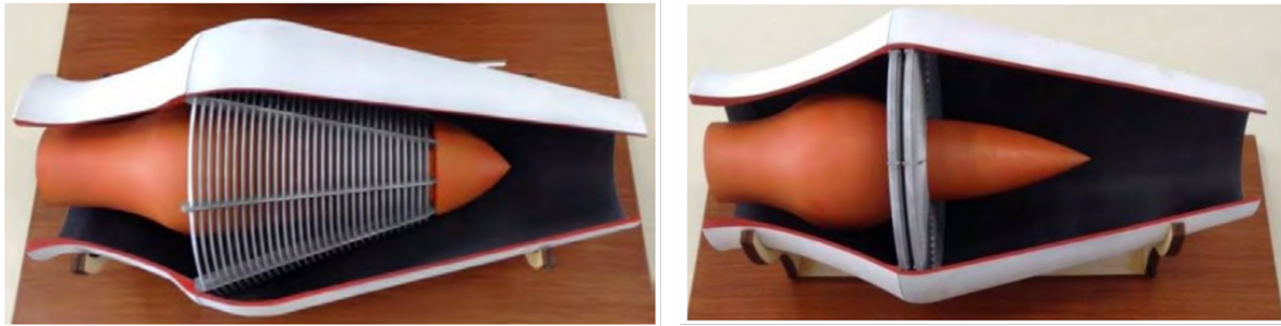
Figure 2.6: The CORN (left) and STARTREC (right) recuperator concepts as proposed by Misirlis et al. [36]
