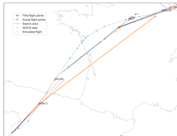
Figure E.2: flight 218929651 towards EDDF. This flight contains no datapoints over the bay of Biscay. Here two turns should be made when looking at the actual flight point (light orange line with dots). Since these turns are missing. The next ATC commands was used. This was a direct to LUTAX. Since no flight points were detected right after the turn above France, and this was the furthest when extending the turn.
