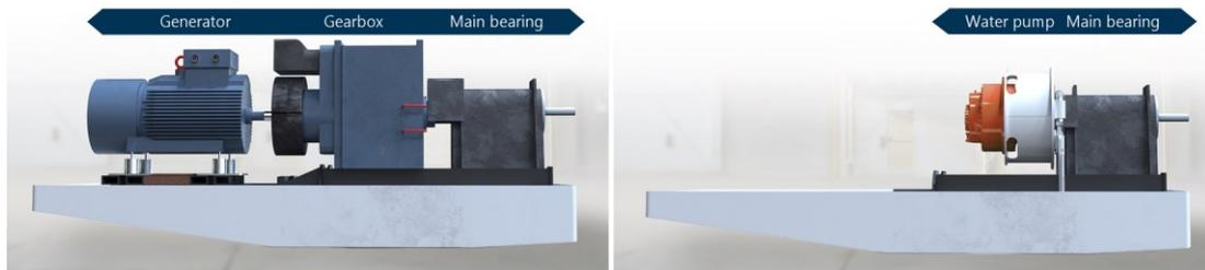
*Figure 1-1: The conventional configuration of a drive-train wind turbine (left) compared to a configuration with hydraulic components (right). The advantage of mass and space reduction in the nacelle is self-evident [12].*
